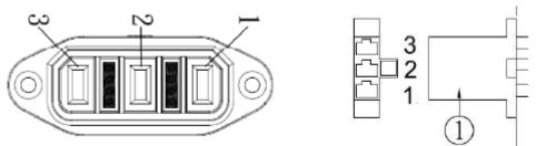
1. Output connector: Sun Shen 3+0pin, DC power connector.
