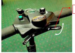
Finger Lever Control/Maximum Force Applied on Lever is 4N
